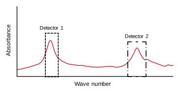
Both observed wavelength ranges and corresponding intensities, are associated with the measured concentration of FAME in the sample, and the result is reported as "FAME in Jet Fuel".
