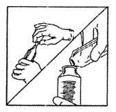
• Cut the shrink seal and pour the saturated Toluene as recommended in API MPMS Chapter 10.3,10.4 and 18.1 into a volumetrically verified centrifuge tube.
