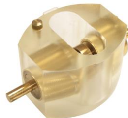
Test Cell: TCDE ASTM D877 (pictured left)
