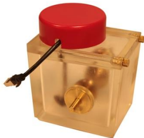
Test Cell: TCVDE ASTM D1816 (pictured left)
