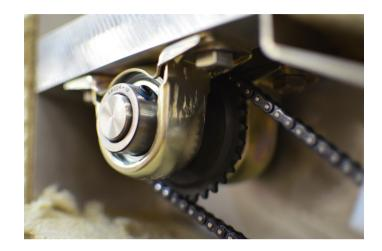
Sealed high temp bearings located outside of heat zone for zero maintenance & durability.
