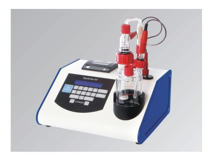
The Aquamax KF Plus titrators have been specifically designed for the determination of water content, combining coulometry with the Karl Fischer method.
