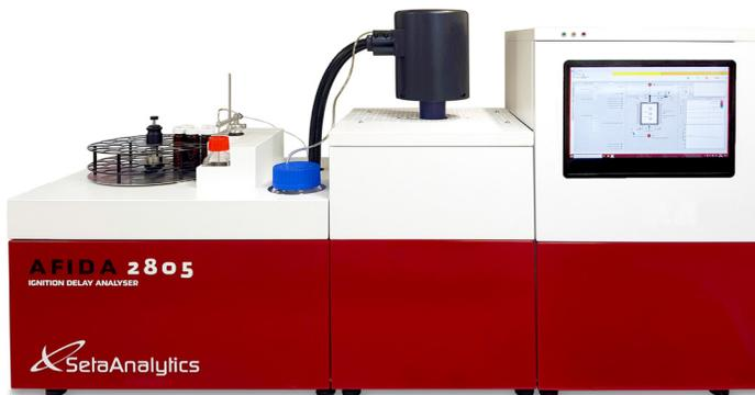
AFIDA is a revolutionary development providing fully automated determination of the Indicated Cetane Number (ICN) of diesel and diesel related fuels.
